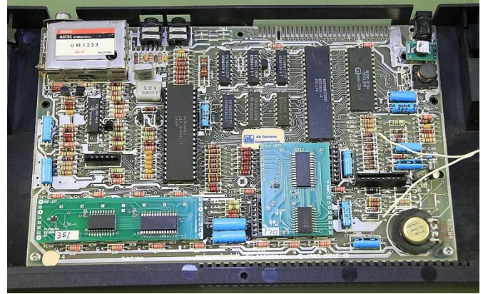
The picture shows the converted ZX Spectrum 48
